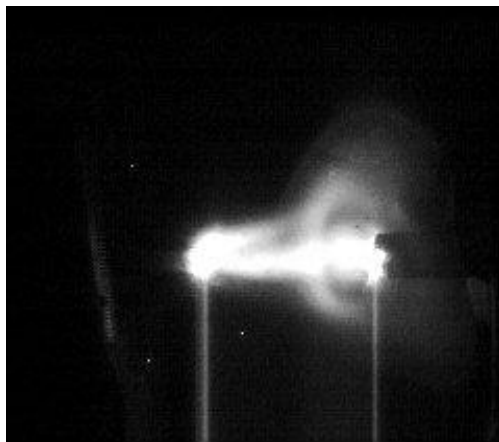
Picture of a self-stable plasma toroid forming around an electric arc
